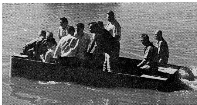
Fig. 22 - The amphibious Spryte vehicle operating in deep water at a speed of 4.5 mph
