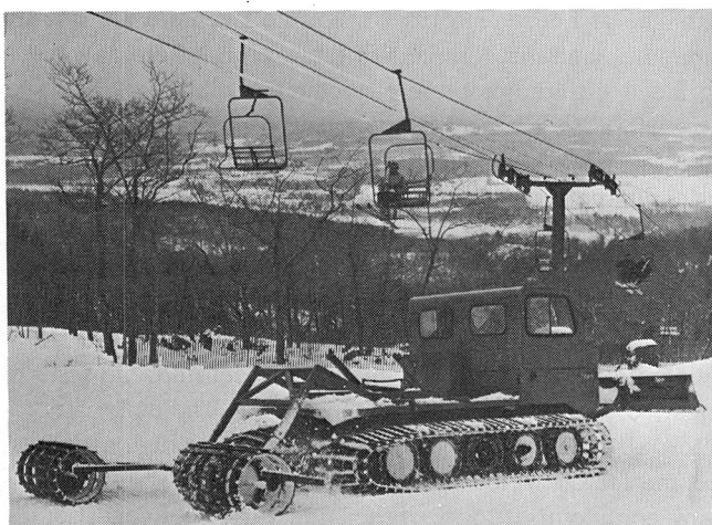
Fig. 4 - Spryte vehicle as equipped for slope grooming work at a ski resort
