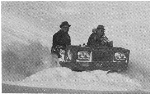
Fig. 9 - Imp vehicle operating in extremely soft powder snow; note snow flowing ahead of vehicle
