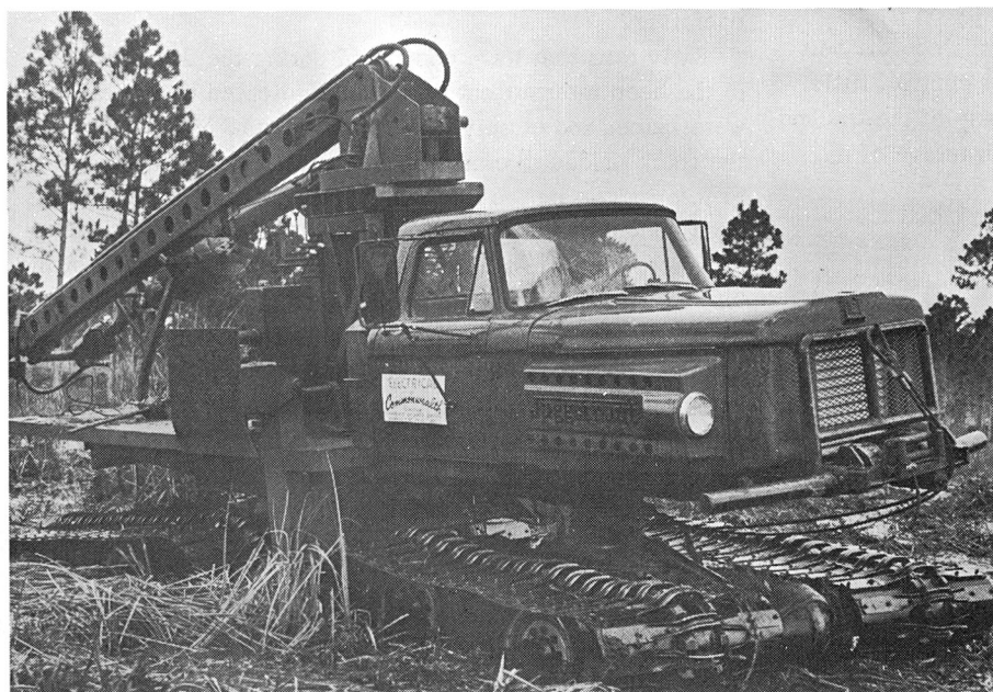
Fig. 28 - Rangemaster vehicle equipped with enclosed planetary steering differential
