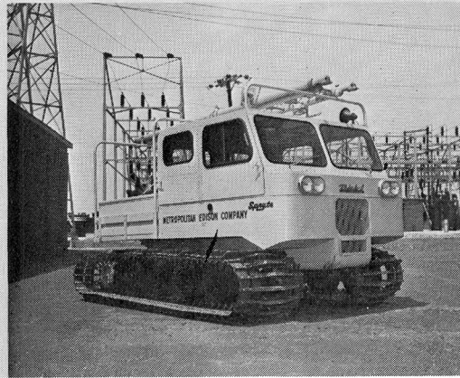
Fig. 1 - Over-snow vehicle as equipped for maintenance work by utility companies
