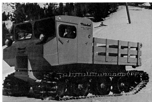
Fig. 8 - Rangemaster vehicle operating on crusted snow surface
