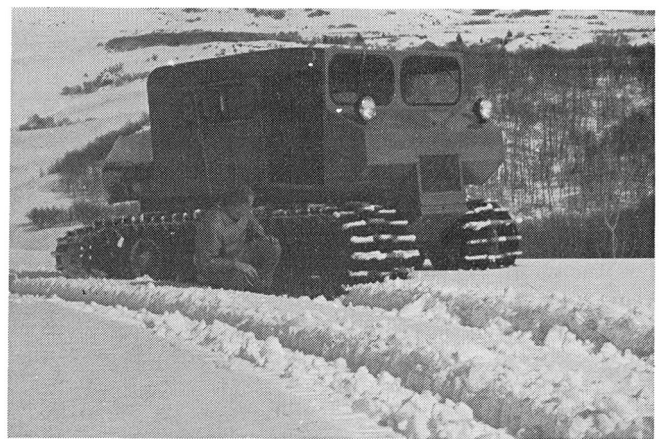
Fig. 11 - Path left by vehicle in packing or snowballing type snow; note definite imprint left by each track cleat
