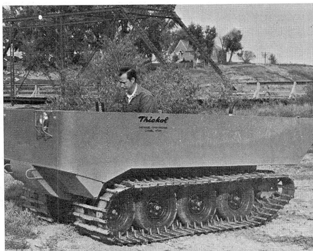
Fig. 21 - Amphibious version of the Spryte over-snow vehicle
