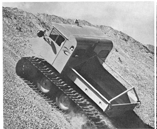
Fig. 16 - Trackmaster vehicle ascending a loose gravel slope at natural angle of repose
