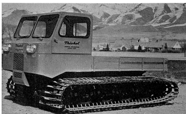
Fig. 25 - Model 1201 Spryte vehicle showing the low sprocket location at rear of vehicle
