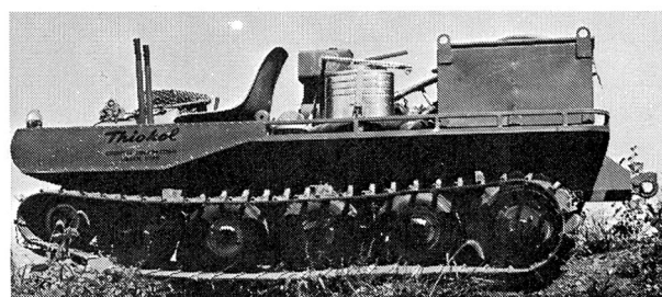
Fig. 26 - Imp vehicle showing the drive sprocket located with the pitch line of sprocket at ground level
