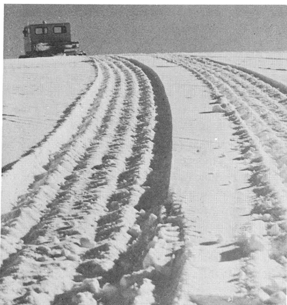
Fig. 10 - Unstructured or nonpacked path left behind the vehicle in sugary snow
