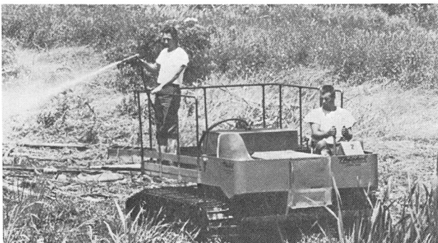
Fig. 19 - The Spryte vehicle spraying for mosquitoes in swampy area
