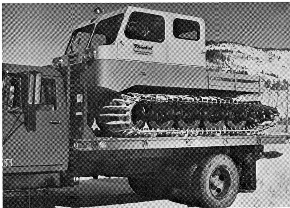
Fig. 2 - Spryte over-snow vehicle loaded for transport to the snow line
