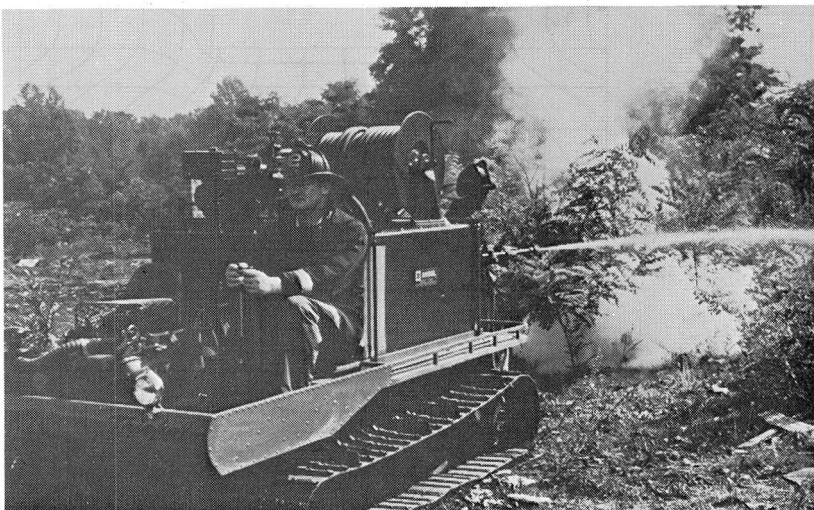
Fig. 14 - Spryte over-snow vehicle ascending steep dirt slopes on fire fighting service in Southern California
